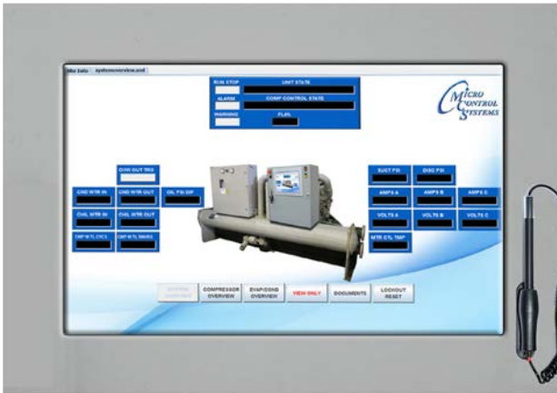
Trane RTHA System Overview
